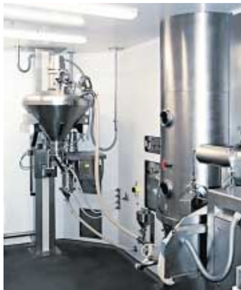
PCS 400 incl. docked sieve GS 180 integrated in a granulation suite
