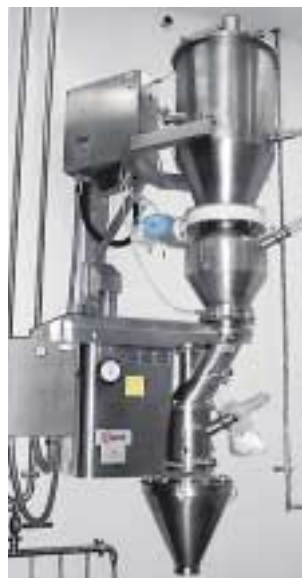
Product separator with buffer vessel and attached rotor sieve GS 180
