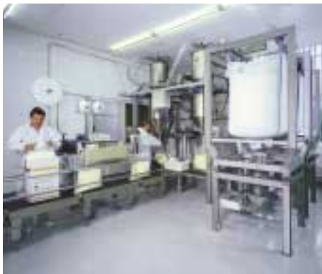
Packing and final wrapping by means of pneumatic conveying system
