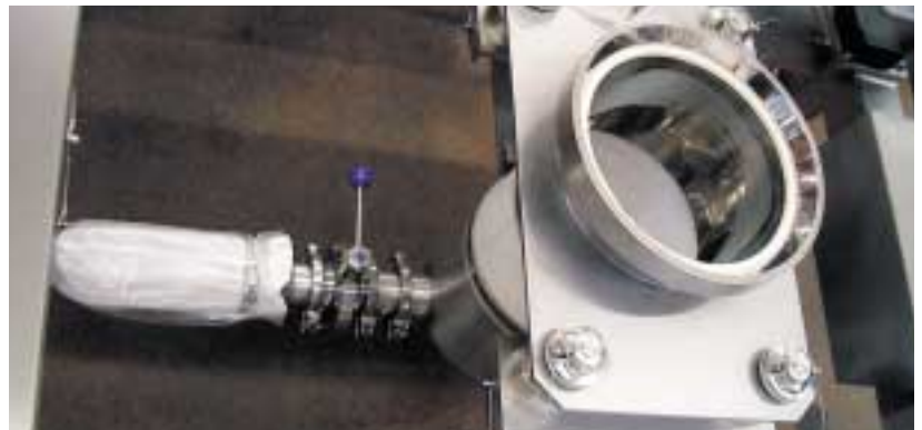
Suction shoe incl. secondary air filter built in an IBC discharge station
